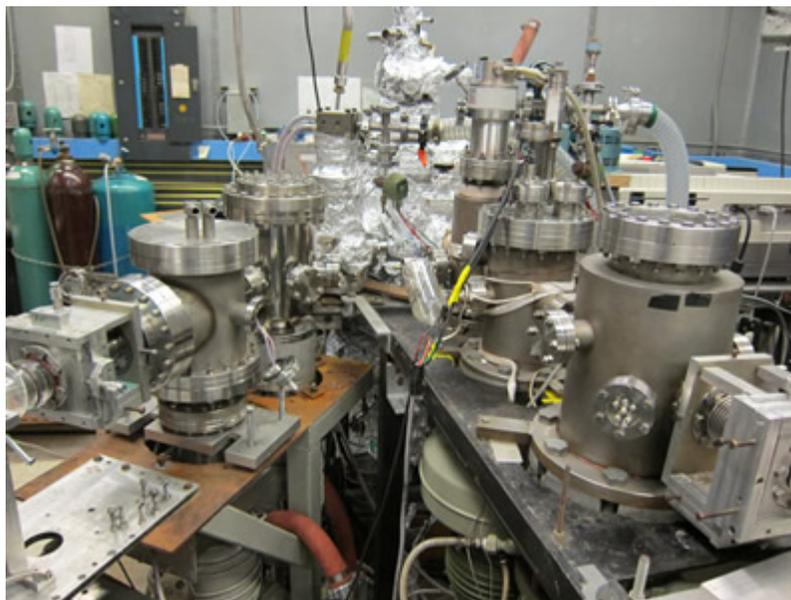
Vidali's team simulates interstellar conditions with a water-cooled, radio-frequency dissociation unit, shown here. The apparatus contains a mass spectrometer that produces charged particles for chemical analysis
